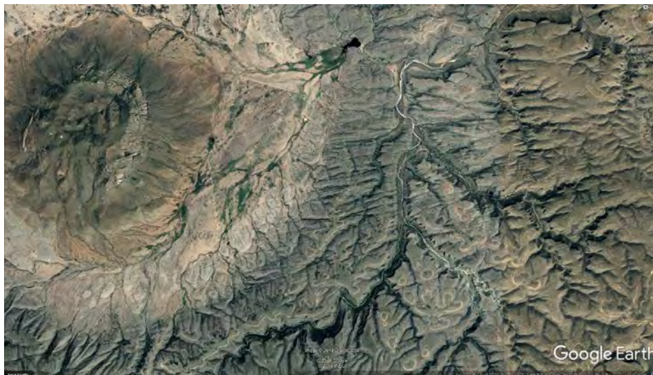
Figure B-9. Drainage and fracture patterns around Tertiary volcanic intrusions southwest of Amistad Reservoir in Coahuila, Mexico
