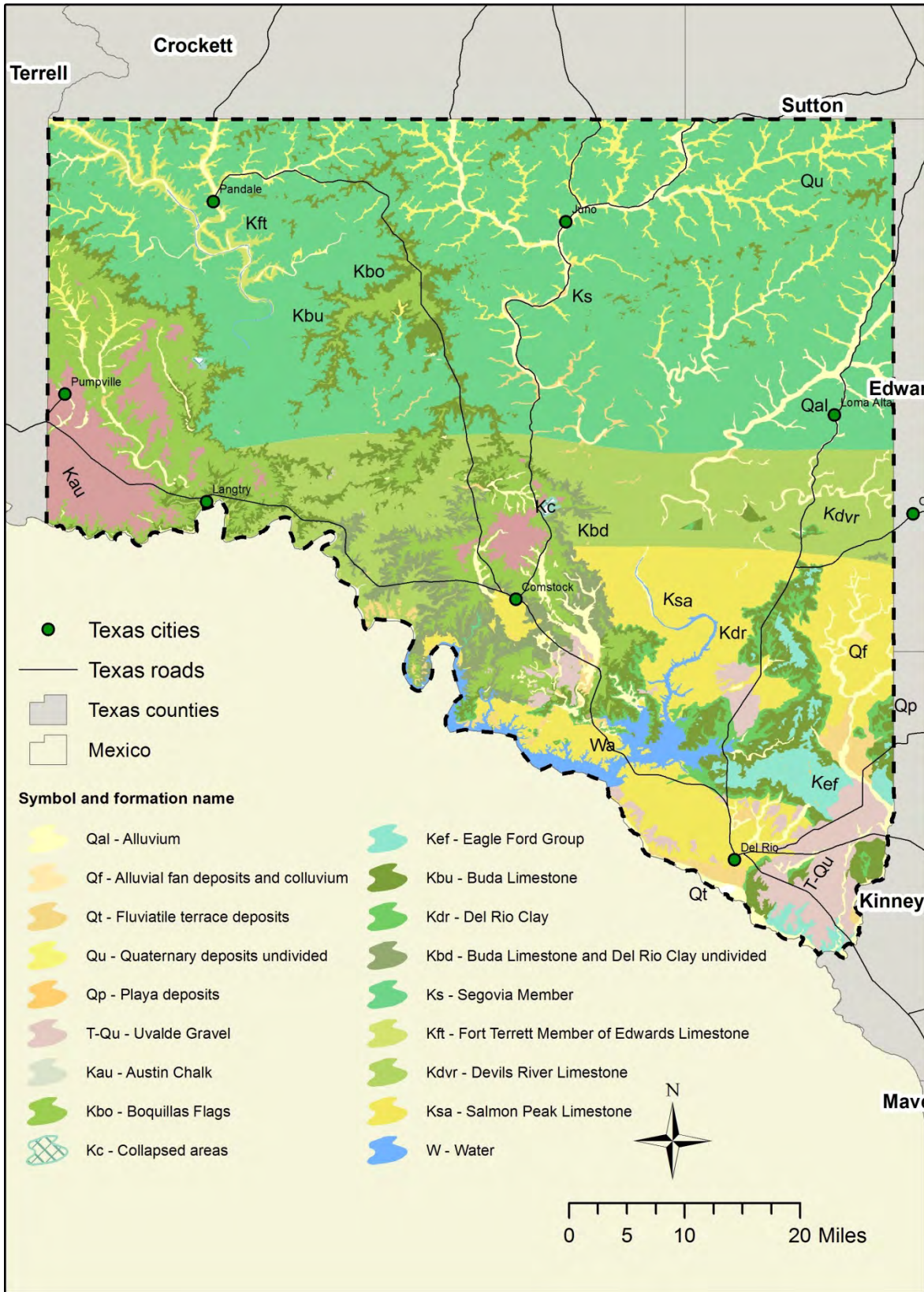
Figure 3-1. Surficial geology of Val Verde County. Modified from the Geologic Atlas of Texas.
